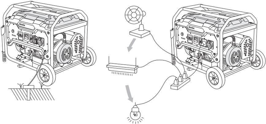
Don't move the earth wire during normal maintenance or repair.
