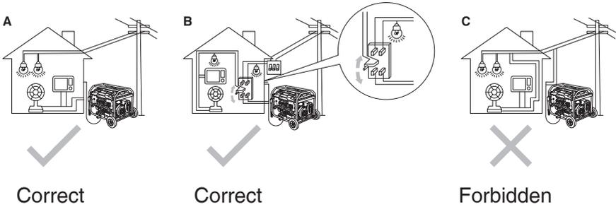
When connect the generator home power supply, be sure that a skilled electrician dose this job. Improper connecting between the generator and loads may cause damage to the generator, even a fire.
