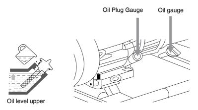
When the oil level is lower than the minimum safety limit, the oil alarm system will automatically stop the engine. To avoid the inconvenience caused by accidents, please check the oil level regularly.
